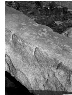
Characteristic marking of feather and wedging on a piece of granite at the site.
